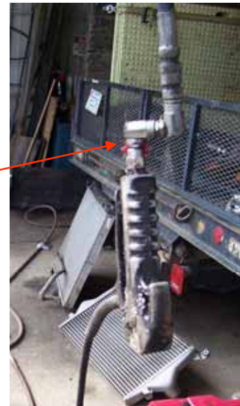
Leaking Handle and swivel
